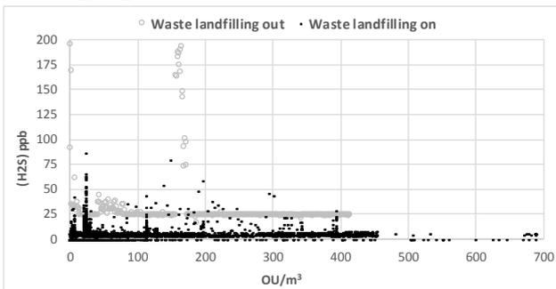
Figure 4: Absence of correlation between H<sub>2</sub>S continuous measurements by the Jerome J605 analyzer and OU/m<sup>3</sup> values obtained by MSEM-32 e-nose with appreciable S-SE wind + calms.
