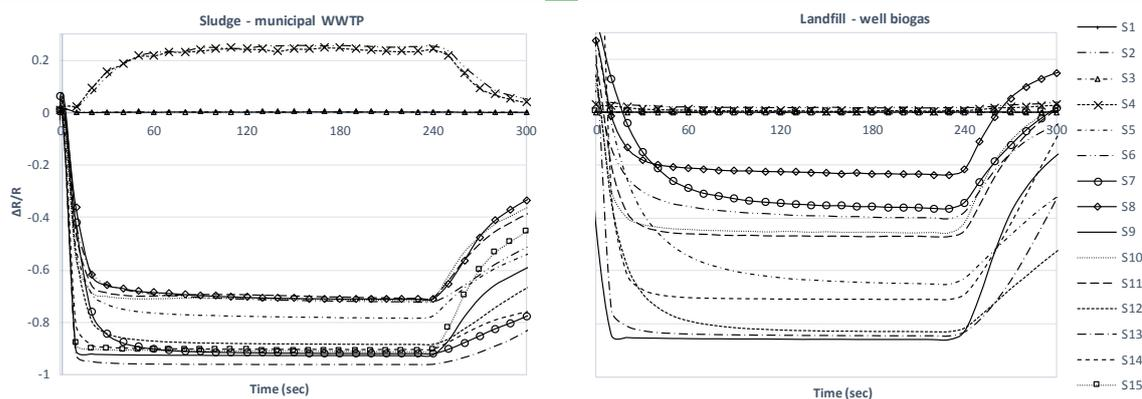
Figure 2: Response of MSEM32 e-nose sensors to the odour classes associated to different sources. There are shown only the sensors with a high value of  $\Delta R/R$ : the sensor response for each time point is calculated as  $(R_t - R_0)/R_0$ , where  $R_0$  is the initial resistance value. Hence the initial datum has  $\Delta R/R = (0 - R_0)/R_0 = 0$ . The time 0 sec corresponds to the start of the odour sampling by the e-nose.
