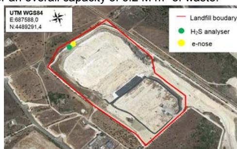
Figure 1b: sanitary landfill and monitoring points
