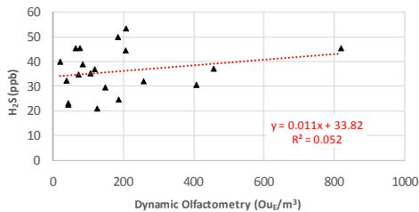
Figure 7: Absence of correlation between H<sub>2</sub>S continuous measurements by Jerome J605 analyzer and OU<sub>E</sub>/m<sup>3</sup> values obtained by dynamic olfactometry
