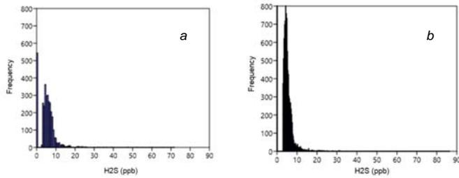
Figure 5: Different probability distributions of H<sub>2</sub>S (ppb) measured by Jerome J605 continuous analyzer, in correspondence of SSE wind and calms (a: Waste landfilling on; b: Waste landfilling out).
