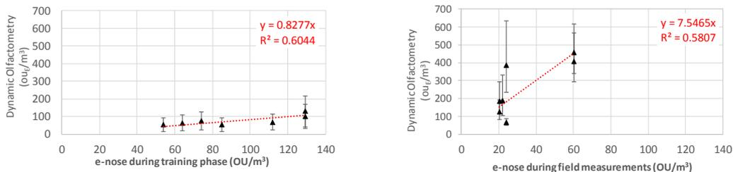
Figure 8. Correlation between OU/m<sup>3</sup> values obtained by the dynamic olfactometry and the e-nose.
